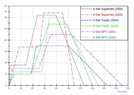
Figure 3 - Simplified deceleration pulses (B pillar) from various EuroNCAP tests (2000 to 2006
