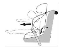
Figure 1: Illustration of lap belt syndrome or submarining.
