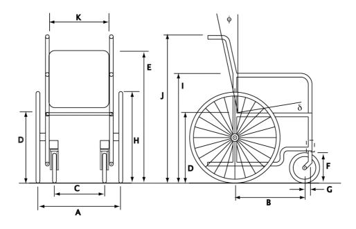
Figure D.1 Critical surrogate manual wheelchair dimensions
