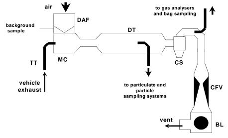
1.4.2. Figure 7: Critical-Flow Venturi Dilution System
