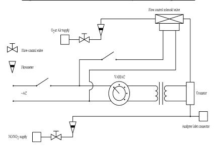
Figure 11: NOx Converter Efficiency Test Configuration
