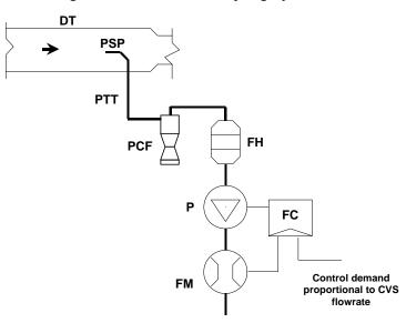
A sample of the diluted exhaust gas is taken from the full flow dilution tunnel DT through the particulate sampling probe PSP and the particulate transfer tube PTT by means of the pump P. The sample is passed through the particle size pre-classifier PCF and the filter holder(s) FH that contain the particulate sampling filter(s). The flow rate for sampling is set by the flow controller FC.
