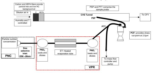
Figure 13: Schematic of Particle Sampling System
