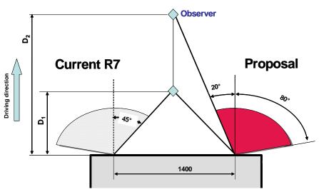
This angular modification allows more pedestrian-friendly front ends. It helps improving the aerodynamics of the vehicle, thus reducing the fuel consumption.
