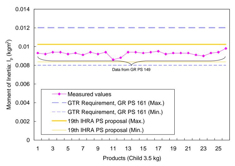
Ip: The moment of inertia about an axis through the centre of gravity and perpendicular to the direction of impact.
