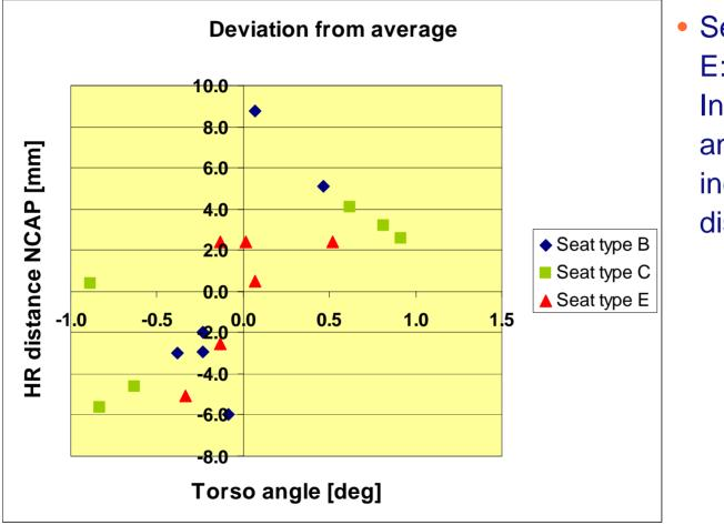
Seat B, C and E: Increasing angle ~ increasing HR distance
