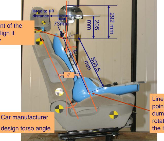
Line through Hpoint of the dummy and rotation point of the HRMD
