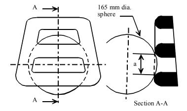
Figure 4-1 - Measurement of a vertical gap "a".
