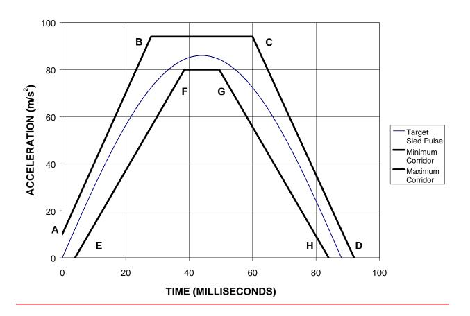
Figure 8.1 - Sled pulse acceleration corridor. The target acceleration with time expressed in milliseconds is a =  $86 \sin(\pi t/88) \text{ m/s}^2$ , for V =  $17.3 \pm 0.6 \text{ km/h}$ . The time zero for the test is defined by the point when the sled acceleration achieves 2.5 m/s<sup>2</sup> (0.25 G's).
