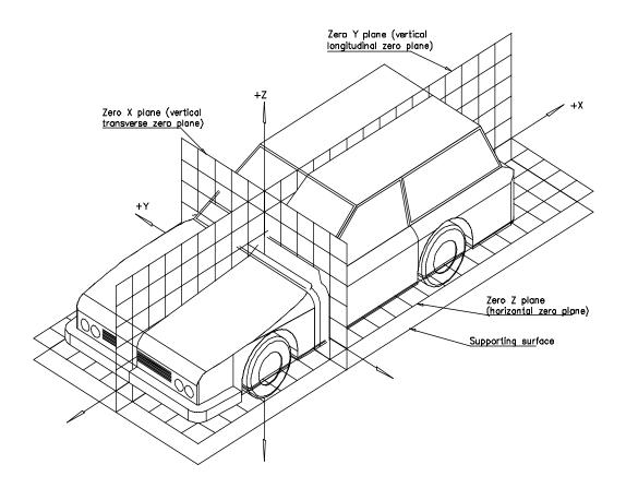
Figure 10-1 - Three-dimensional reference system
