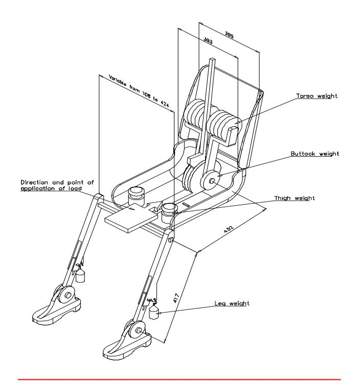
Figure 11-2 - Dimensions of the 3-D H machine elements and load distribution (Dimensions in millimeters)
