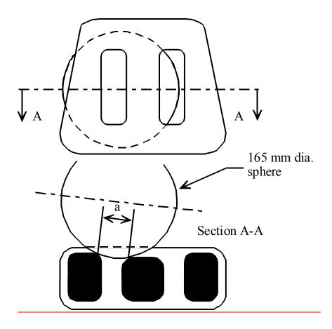
Figure 4-2 - Measurement of a horizontal gap "a".
