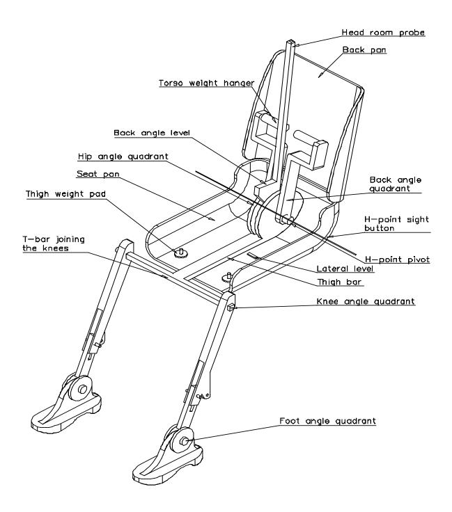
Figure 11-1 - 3-D H machine elements designation
