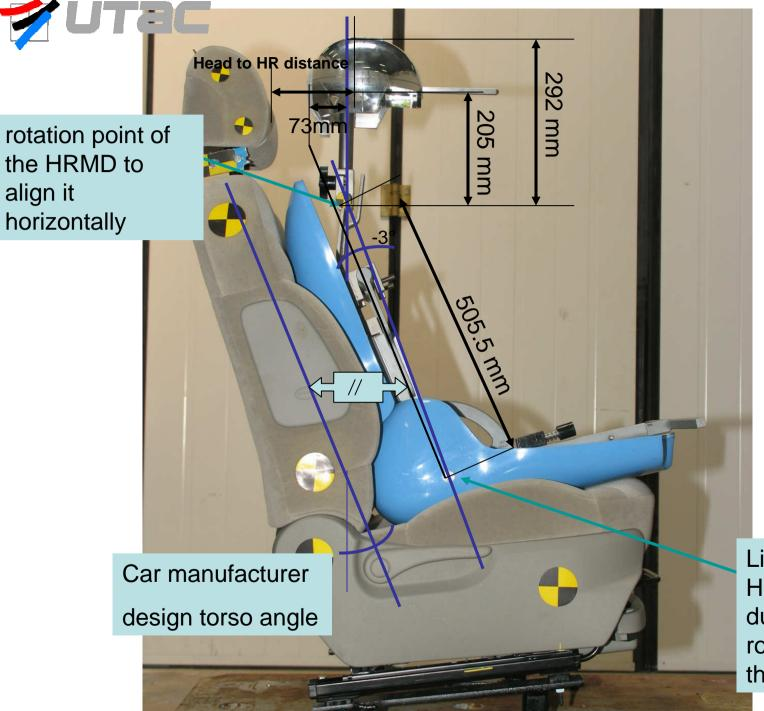
Line through Hpoint of the dummy and rotation point of the HRMD
