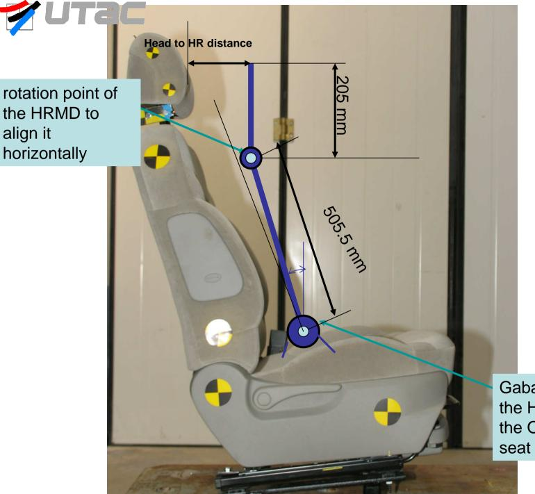
Gabarit adjust at the H point and at the OEM design seat angle
