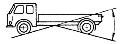
4.7.3.4. "Ground clearance between the axles" means the shortest distance between the ground plane and the lowest fixed point of the vehicle.
