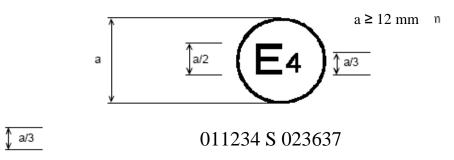
The above approval mark shows that the tyre concerned has been approved in the Netherlands (E4) pursuant to Regulation No. 117 (marked by S (rolling sound), under approval number 011234 and Regulation 30 under approval number 023637. The first two digits of the approval number (01) indicate that the approval was granted according to the 01 series of amendments, but Regulation No. 30 included the 02 series of amendments.
