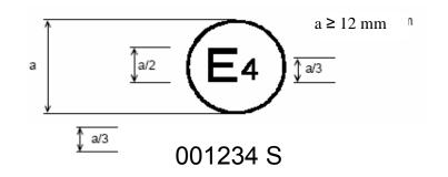
The above approval mark, affixed to a pneumatic tyre shows that a tyre concerned has been approved in the Netherlands (E4) pursuant to Regulation No. 117 (marked by S (rolling sound) only), under approval number 001234. The first two digits of the approval number (00) indicate that the approval was granted according to the requirements of this Regulation in its original form.
