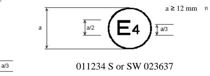
The above approval mark shows that the tyre concerned has been approved in the Netherlands (E4) pursuant to Regulation No. 117 (marked by S (rolling sound) or SW (rolling sound and wet adhesion), under approval number 011234 and Regulation 30 under approval number 023637. The first two digits of the approval number (01) indicate that the approval was granted according to the 01 series of amendments, but Regulation No. 30 included the 02 series of amendments.
