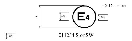
The above approval mark shows that the tyre concerned has been approved in the Netherlands (E4) pursuant to Regulation No. 117 (marked by S (rolling sound) or both S (rolling sound) and W (wet adhesion), under approval number 011234. This indicates that the approval is for S or both SW. The first two digits of the approval number (01) indicate that the approval was granted according to the 01 series of amendments.
