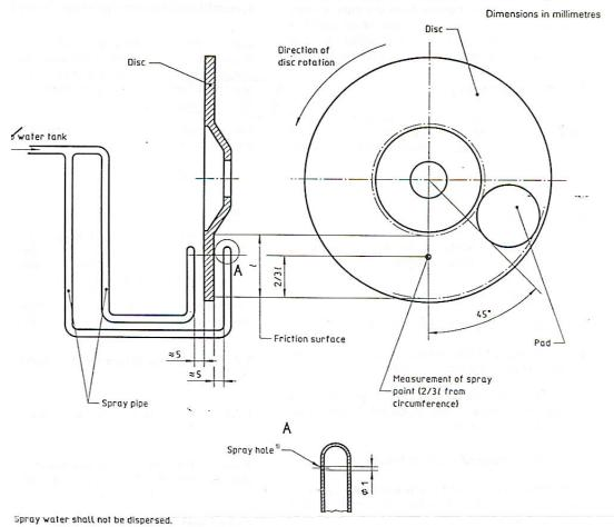
The disc brake water spray equipment shall be is installed as follows:
