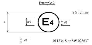
The above approval mark shows that the tyre concerned has been approved in the Netherlands (E4) pursuant to Regulation No. 117 (marked by S (rolling sound) or SW (rolling sound and wet adhesion)), under approval number 011234 and Regulation No. 30 under approval number 023637. The first two digits of the approval number (01) indicate that the approval was granted according to the 01 series of amendments, but Regulation No. 30 included the 02 series of amendments.
