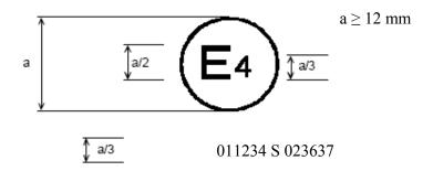
The above approval mark shows that the tyre concerned has been approved in the Netherlands (E4) pursuant to Regulation No. 117 (marked by S (rolling sound)), under approval number 011234 and Regulation No. 30, under approval number 023637. The first two digits of the approval number (01) indicate that the approval was granted according to the 01 series of amendments, but Regulation No. 30 included the 02 series of amendments.
