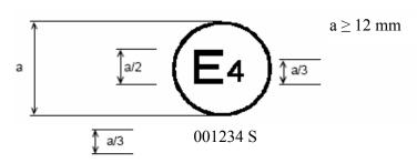
The above approval mark, affixed to a pneumatic tyre shows that a tyre concerned has been approved in the Netherlands (E4) pursuant to Regulation No. 117 (marked by S (rolling sound) only), under approval number 001234. The first two digits of the approval number (00) indicate that the approval was granted according to the requirements of this Regulation in its original form.
