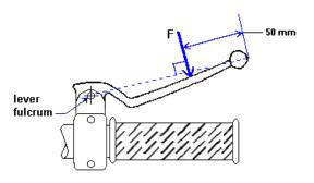
The input force is applied to a point located 50 mm from the outermost point of the control lever, measured along the axis between the central axis of the fulcrum of the lever and its outermost point.
