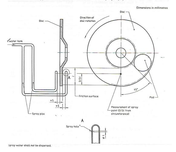
The disc brake water spray equipment is installed as follows:
