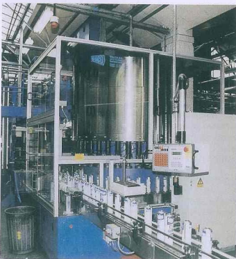
Rotary can tester installed in an aerosol can production line
