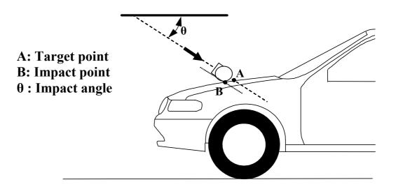
Figure 6: Impact Pointpoint. (insertion of impact angle example) (see §3.17. and §3.24.)
