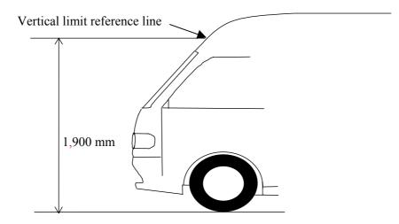
Figure 10: Vertical Limit-limit Reference-reference Lineline. (see §3.30.)
