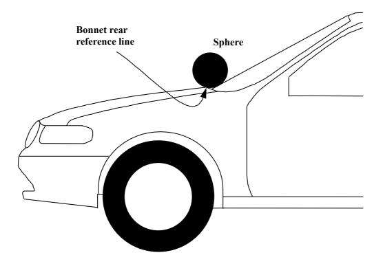
Figure 2: Bonnet Rear-rear Reference-reference Lineline. (see §3.7.)
