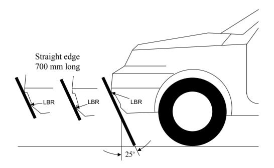
Figure 7: Lower Bumper bumper Reference reference Lineline. (see §3.19.)
