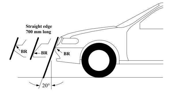
Figure 9: Upper Bumper bumper Reference reference Lineline. (see §3.28.)
