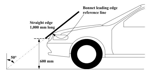
Figure 1: Bonnet Leading leading Edge edge Reference reference Lineline. (see §3.6.)
