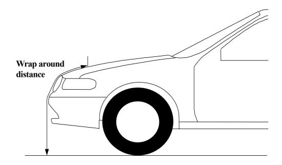
Figure 11: Wrap Around around Distance distance Measurement (see §3.31.)
