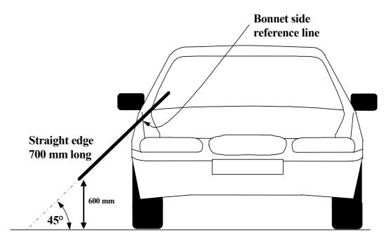
Figure 8: Side Reference reference Lineline. (see §3.23.)
