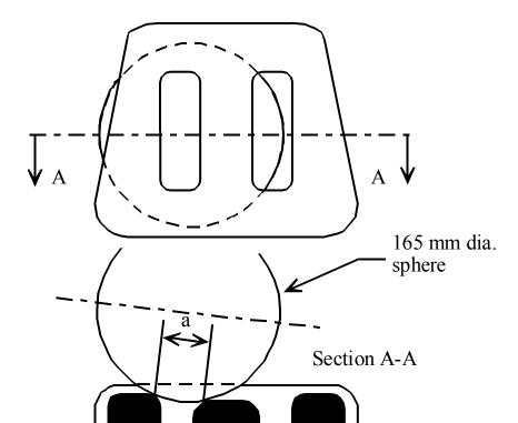
Figure 3 - Measurement of a horizontal gap "a".
