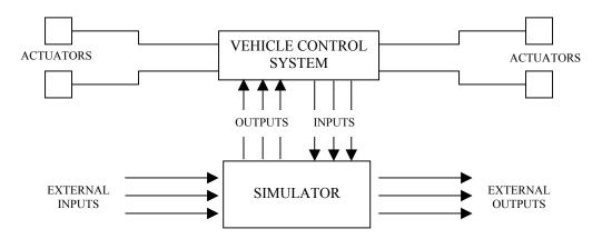
1.3. The simulator shall at least include the following parameters:
