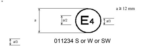
The above approval mark shows that the tyre concerned has been approved in the Netherlands (E4) pursuant to Regulation No. 117 (marked by S (rolling sound) or W (wet adhesion) or both SW), under approval number 011234. This indicates that the approval is for S (rolling sound), W (wet adhesion) or both SW. The first two digits of the approval number (01) indicate that the approval was granted according to the 01 series of amendments."
