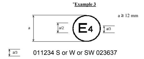
The above approval mark shows that the tyre concerned has been approved in the Netherlands (E4) pursuant to Regulation No. 117 (marked by S (rolling sound) or W (wet adhesion) or both SW), under approval number 011234. This indicates that the approval is for S (rolling sound), W (wet adhesion) or both SW. The first two digits of the approval number (01) indicate that the approval was granted according to the 01 series of amendments, but Regulation No. 30 included the 02 series of amendments."
