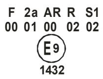
The above example corresponds to the marking of a lens intended to be used in different types of lamps. The approval marks indicate that the device was approved in Spain (E9) under approval number 1432 and comprises:
