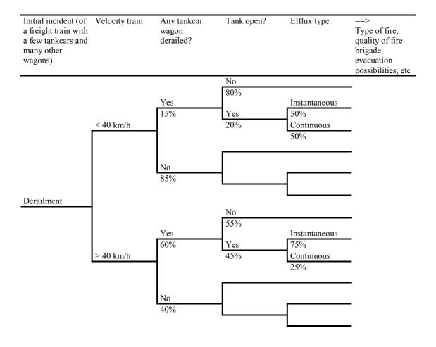
**Figure 3**: Example of a section of an **fault** event tree for a rail tank-wagon for inflammable liquids. The quantitative values are arbitrary.
