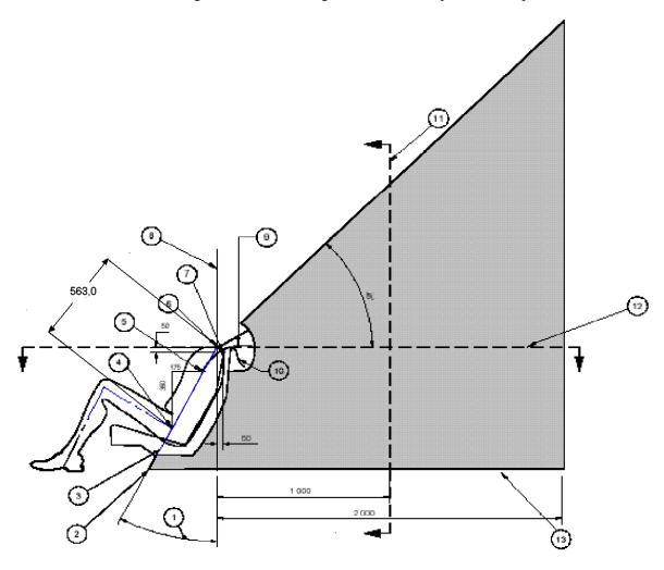
Insert a new dimensioning of 563.0 mm in figure 6 between R point and H point:
