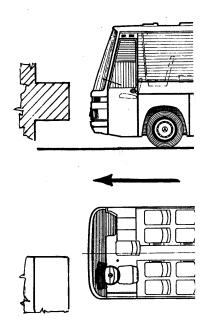
2.3. Collision on the service door side with HPO
