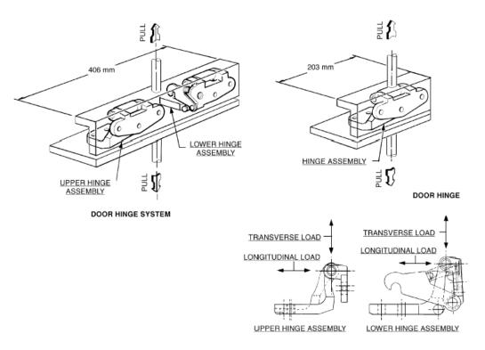
Figure 3-1 – Static test fixtures
