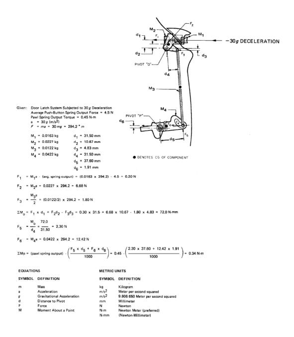
Figure 2-1 – Inertial Loading – Sample Calculation
