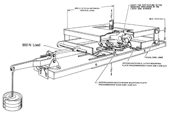
Figure 1-1 – Door Latch - Tensile Testing Fixture for Load Test 1
