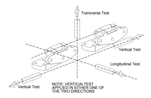
Figure 3-2 – Static load test directions for back doors
