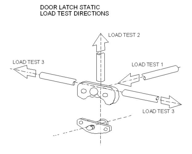
Figure 1-4 – Door Static Load Test Directions
