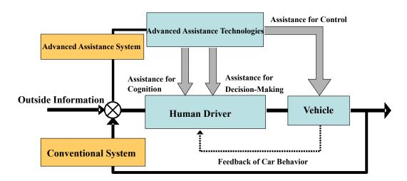
Figure 1 Block Diagram of Car Driving
