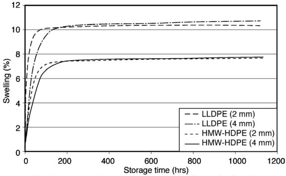
Fig 5 Swelling of HMW-HDPE and LLDPE material as a function of storage time for 2 thicknesses in xylene mixture at  $40^{\circ}$ C
