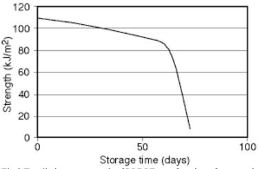
Fig 2 Tensile impact strength of LLDPE as a function of storage time in nitric acid 55% at 40°C
