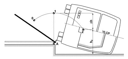
Figure A7.A1.2 - Determination of the vertical movement of the vehicle centre of gravity
