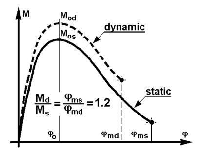
Figure A8. 1A. 2 - Derivation of plastic hinge dynamic characteristics from the static curve
