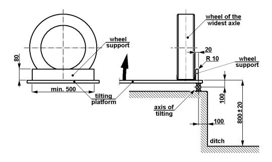
Figure A5.1 - Geometry of the tilting bench
