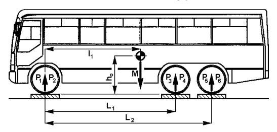
Figure A3.1 - Longitudinal position of the centre of gravity
