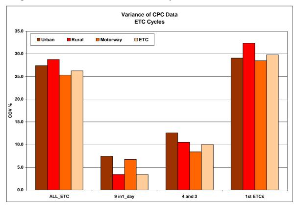
Figure 4 : CPC Measurements over the ETC Cycle - COVs
