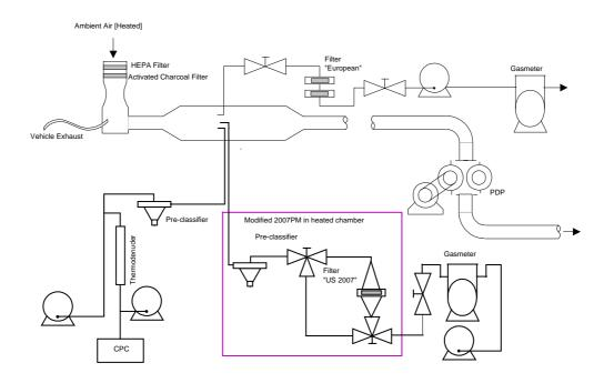
Figure 1a: Indicative Instrument and System Set-up (Light-duty).
