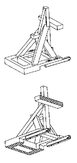
Figure 1: Static force application device (SFAD), isometric views
