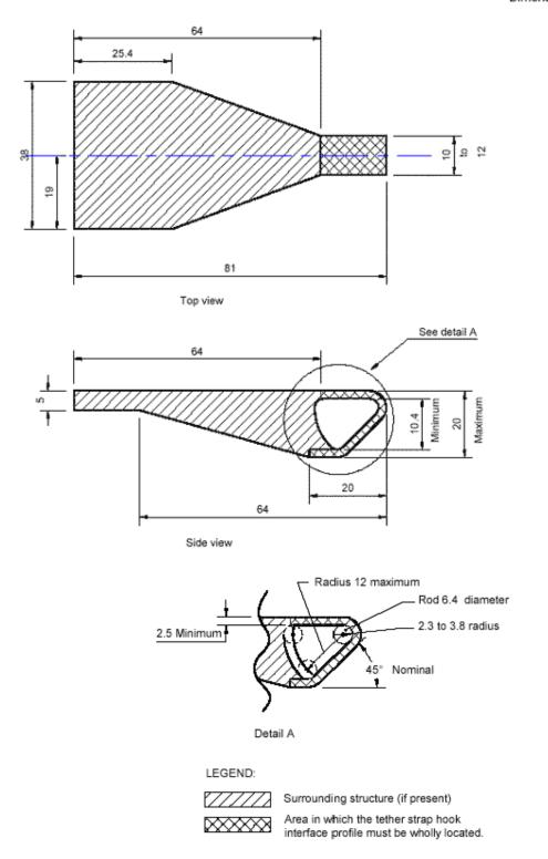
Figure 3: ISOFIX Top tether connector (hook type) dimensions
