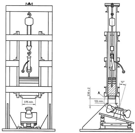
Figure 1 - Impact loading test machine
