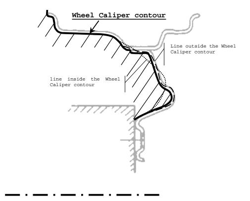
Figure 1: wheel inner contour including examples of inside and outside situations.
