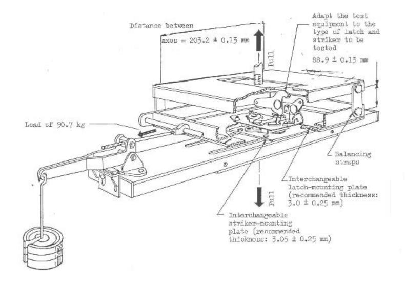
Test procedure for latches: transversal load
