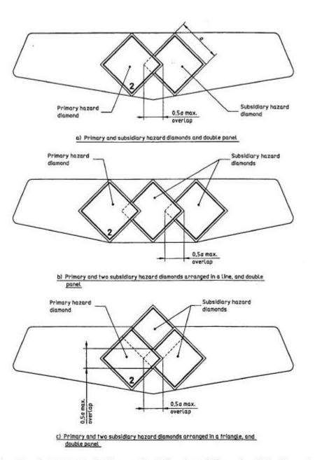
Figure 2 — Arrangements of primary and subsidiary hazard diamonds and double panels
