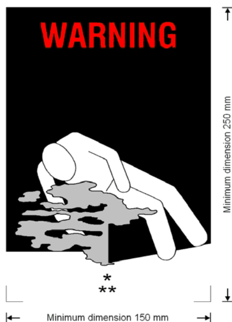
Coolant/conditioning warning mark for cargo transport units
