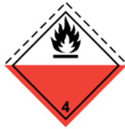
(No. 4.2) Division 4.2 Substances liable to spontaneous combustion Symbol (flame): black; Background: upper half white, lower half red; Figure '4' in bottom corner
