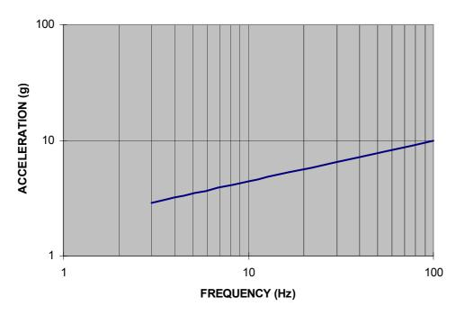
Equation for generating the above Minimum SRS Curve:  $ACCEL = 1.95 FREQ^{0.355}$
