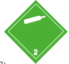
(No. 2.2) Non flammable, non-toxic gases Symbol (gas cylinder): black or white; Background: green; Figure '2' in bottom corner
