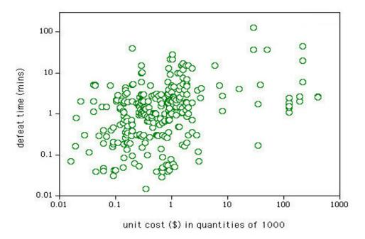
Figure 9 - Seal cost is not a good predictor of vulnerability.
