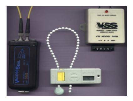
Figure 7 - Three examples of active seals.
