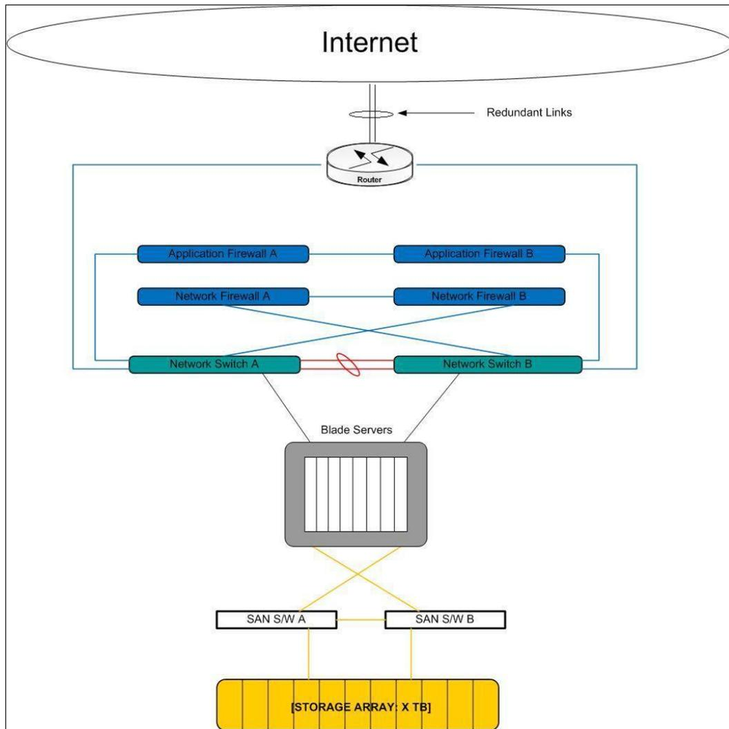
**Figure 2-4: The Blade Center Configuration**
