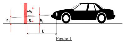
Dipped-beam downward inclination of a category M<sub>1</sub> vehicle
