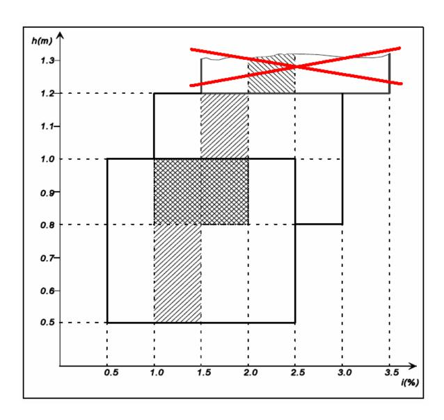
[Moreover, it shall be possible to adjust (the initial aim of) the vertical inclination, without affecting the horizontal aim of the dipped-beam headlamps.]
