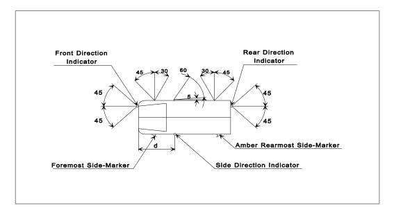
Vertical angles: 15° above and below the horizontal. The vertical angle below the horizontal may be reduced to 5° if the lamps are less than 750 mm above the ground.
