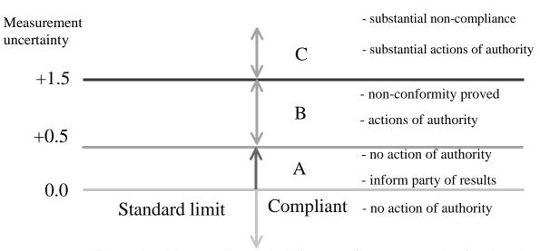
Figure: visualising compliance criteria for a specific test on a product (conducted emission)
