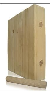
**Notes:** "Brettstapel" board; the plies are held together through long kiln-dried plugs made of beech which are inserted into pre-drilled holes; as soon as they absorb the moisture from the environment they swell leading to a strong bond between the different wooden parts of the board.
