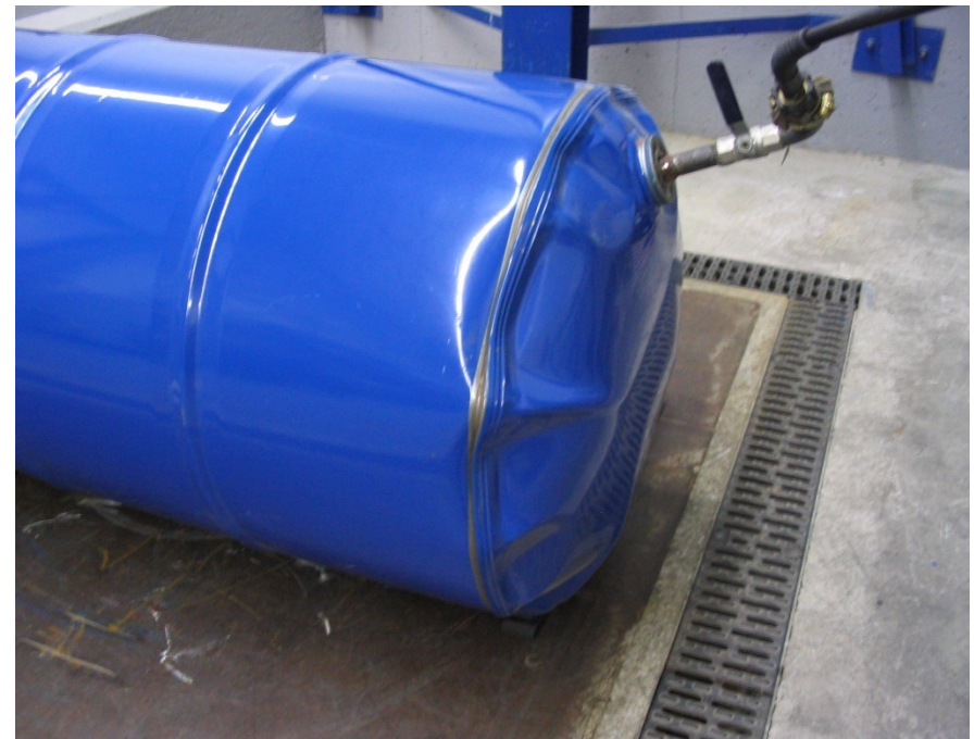
Hydraulic pressure test
