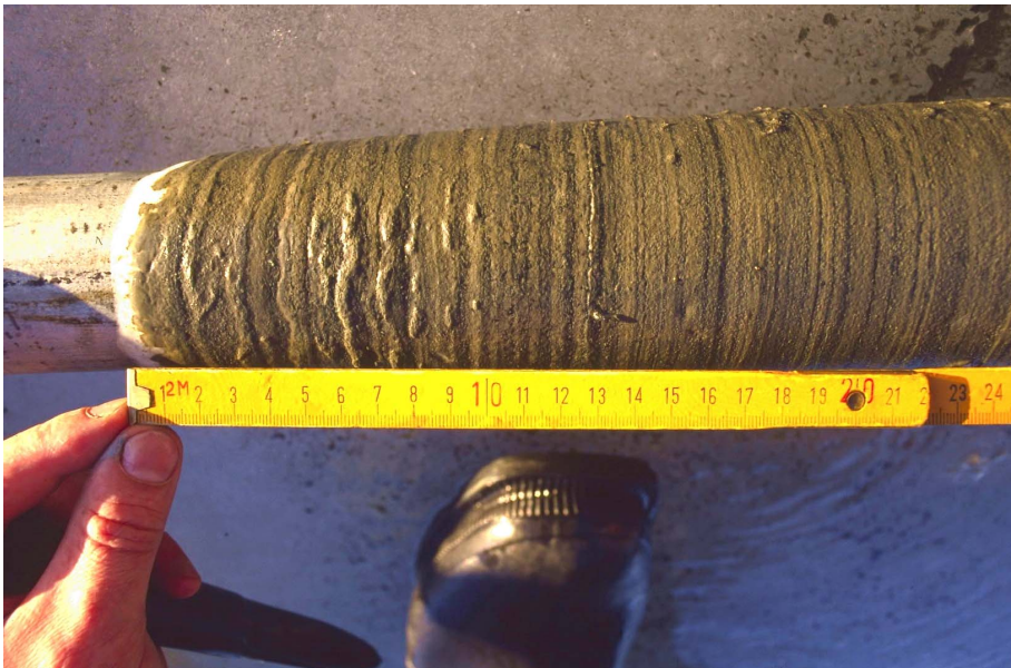
Figure 24. Figure 24. A sediment sample taken with a gravity corer. In this case different layers can be detected easily (Photo Seppo Knuutila).
