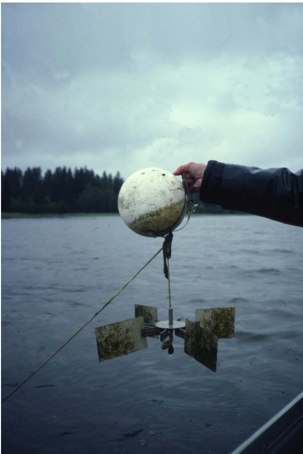
Figure 18. The incubation equipment for estimation of periphytic growth in lakes (Photo Sirpa Herve).
