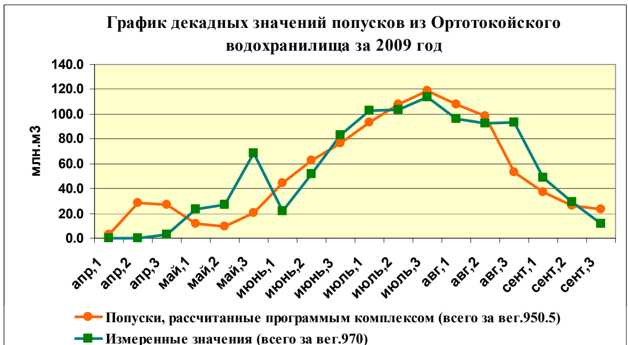
Example of computer calculation of discharges (red graph) from the Orto-Tokoi reservoir on the Chu River in comparison with actual data (green graph)
