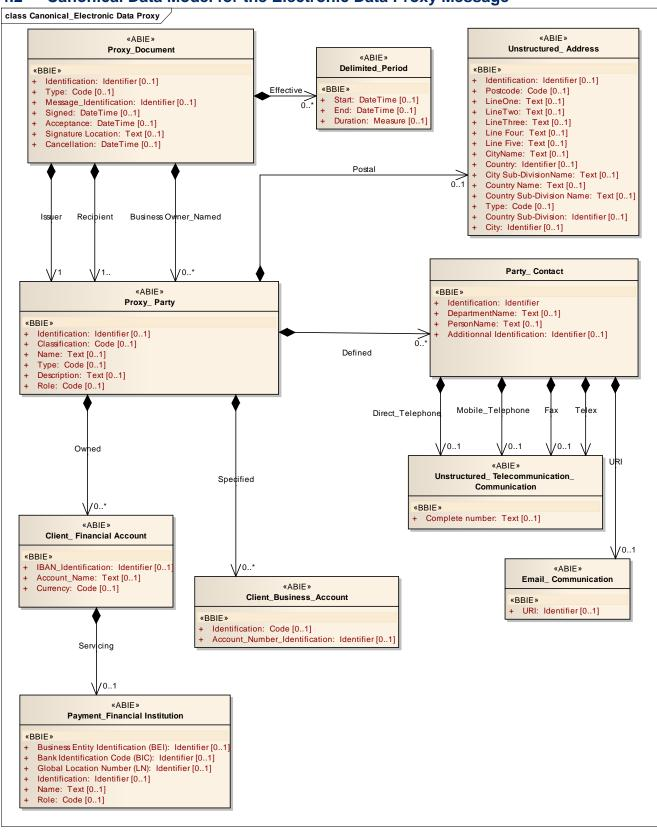
Figure 4-2 Canonical Electronic Data Proxy
